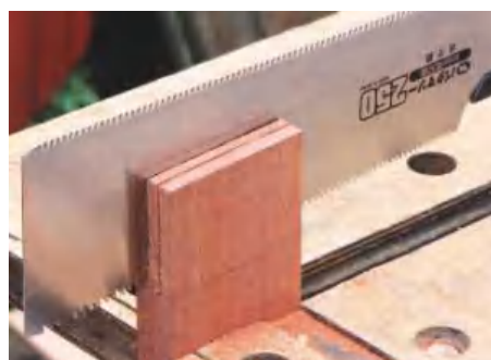
▲ The Ryoba saw is good for cutting tenons and bridle joints
